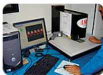
This technician is examining the height of solder paste deposition after stenciling, another critical factor in creating high-quality BGA assemblies.
